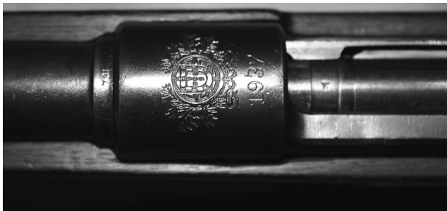
Figure 5.9 The receiver markings of a Model 1937 Short Rifle, the Portuguese designation for the Mauser 98 pattern taken into service in 1937. The 1937 mark indicates the year of production, a standard marking that appears on Model 98 rifles. The emblem is the Portuguese crest and appeared on Model 98 rifles exported to Portugal from Mauser in Germany. (Image from author's collection.)
